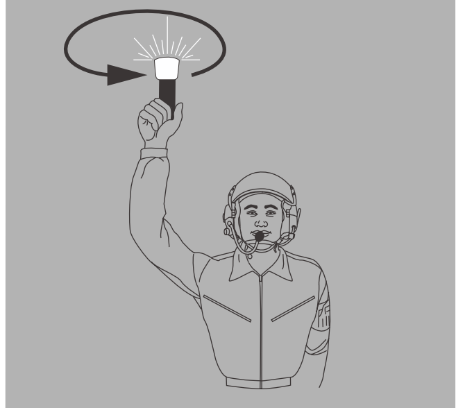
Turn light on when right arm is extended overhead; execute large horizontal circle. Turn light off before lowering arm. Repeat as necessary.
